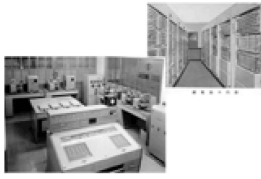
Fujitsu FACOM 128A system with the control console in the foreground (bottom), the system's relay rack (top).
