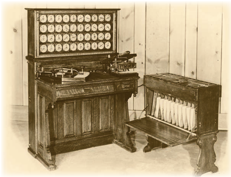
The U.S. Census Bureau used this electromechanical machine, invented by bureau engineer Herman Hollerith, to tabulate statistics for the 1890 census.
