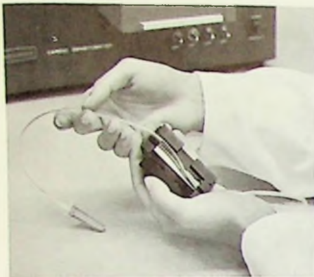
Flow-through cuvette used with dye dilution cardiac output instrument.
