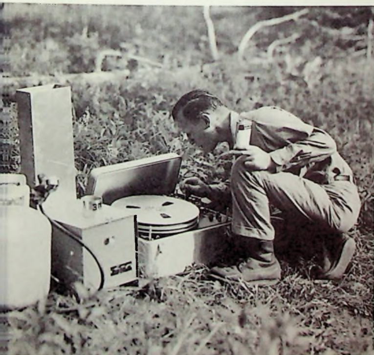
Portable field Seismometer in use as a part of USGS investigations of earthquakes and earth movements.
