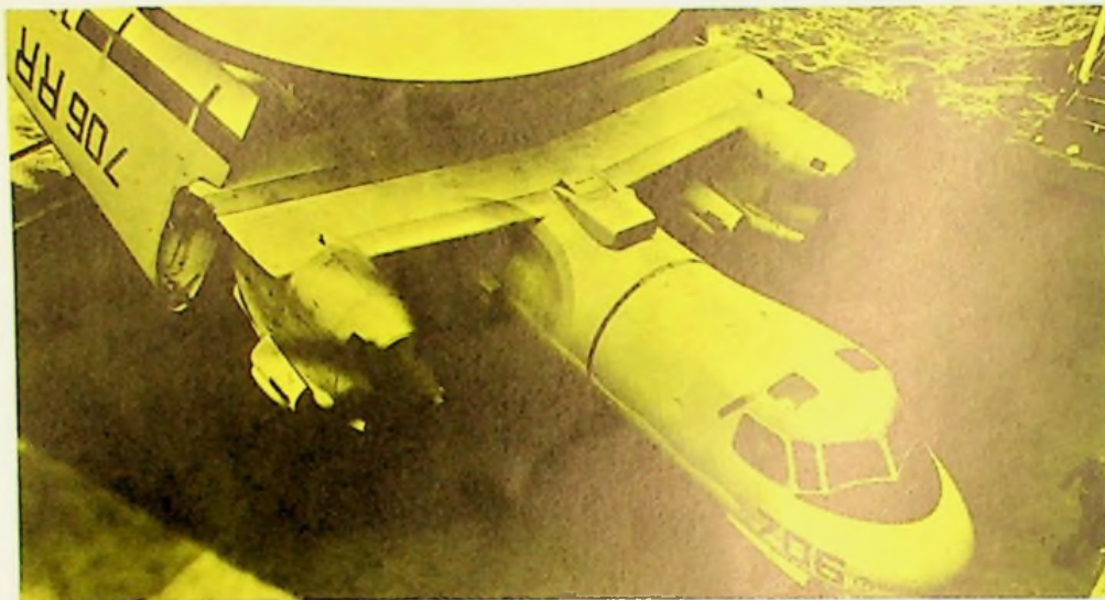
ROTODOME* ANTENNA EXTENDS NAVY'S SEE AT SEA — An AN/APA-143 ROTODOME radar antenna (large disk-shaped structure) is shown mounted atop a Navy E-2A Hawkeye, a Grumman-built carrier-based early warning aircraft.
