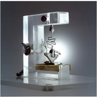
A replica of Bell Labs' first point-contact transistor.
