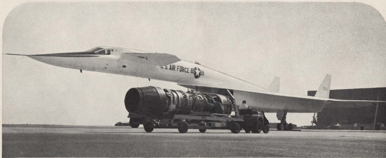
DEFENSE —G-E engineers designed and produced six J93 engines to push USAF XB-70 to Mach 3.
