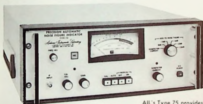
AIL's Type 75 provides automatic noise figure indication from 0 to 33 dB in the RF range from 10MHz to 40 GHz. Price less cabinet: $1500.
