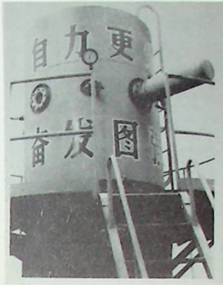
5 MEV VAN DE GRAFF GENERATOR USED FOR NUCLEAR PHYSICS STUDIES IN SHANGHAI, CHINA.
